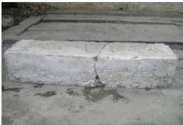
Fig 18: Tested specimens of beam (c)
