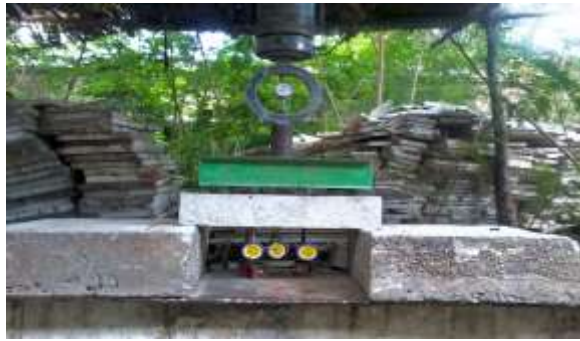
Figure 11: Flexural Strength test setup
